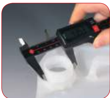
Measuring of canister thread
